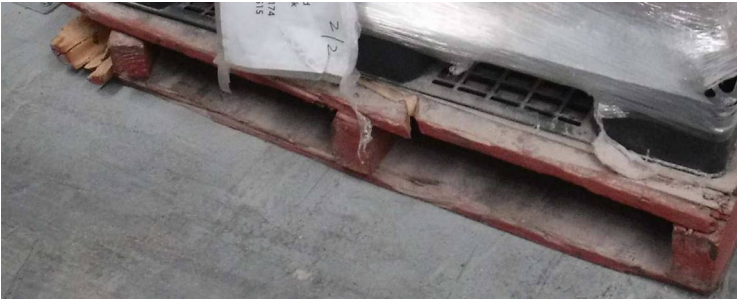
Figure 3: Split stringer at left, damaged front deckboard and visible food residue.
