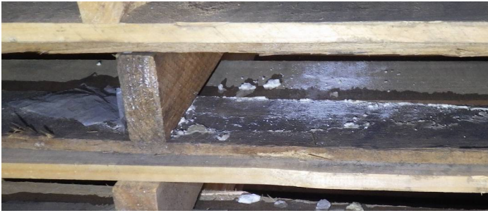
Figure 1: Pallets with white surface deposits, splintering and old attached wrapping
