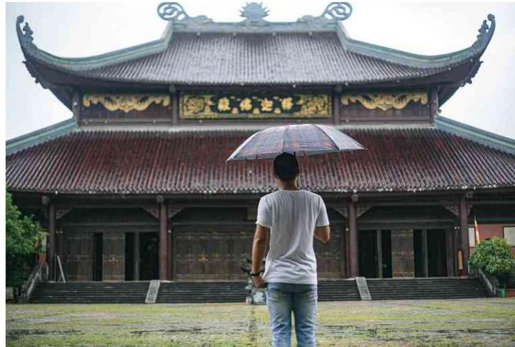
1 As in the pictured pagoda, a good roof will protect the exterior walls and the footings from excess moisture. Ideally, the bottom metre of exterior wall will not be regularly wetted by rains or splashing.
