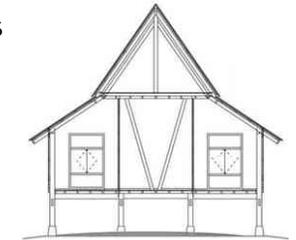
It is not always possible to achieve such elevations. Ideally a suspended floor will sit far enough above the ground that there is always room for an inspector to go fully underneath. No part of the sub-floor area should be fully enclosed so that it becomes inaccessible or lacks natural cross ventilation.
